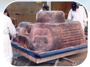
Each layer is hand rolled to eliminate trapped air pockets.
