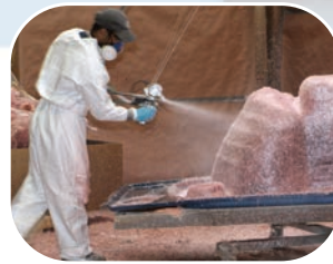
Multiple layers of fiberglass and resin are applied.
